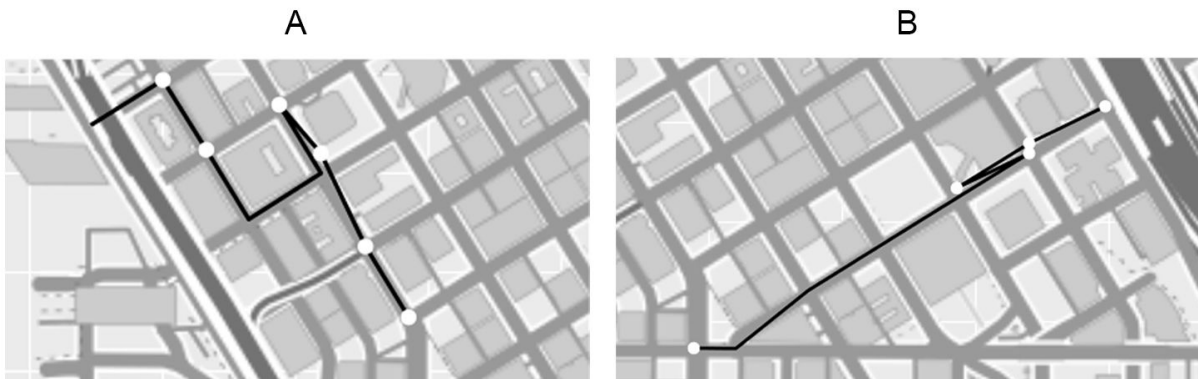
Figure 4. Routing artifacts due to high sensor range
